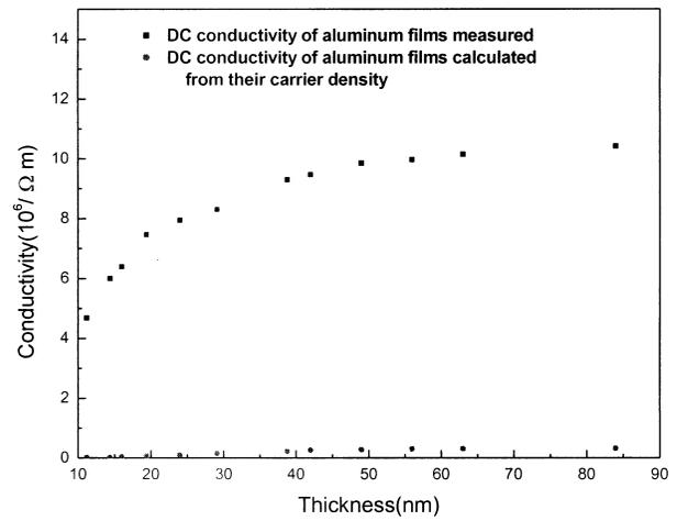
Figure 3 Comparison of ultrathin aluminum films on DC conductivity between measured value and calculated value from their carrier density.
