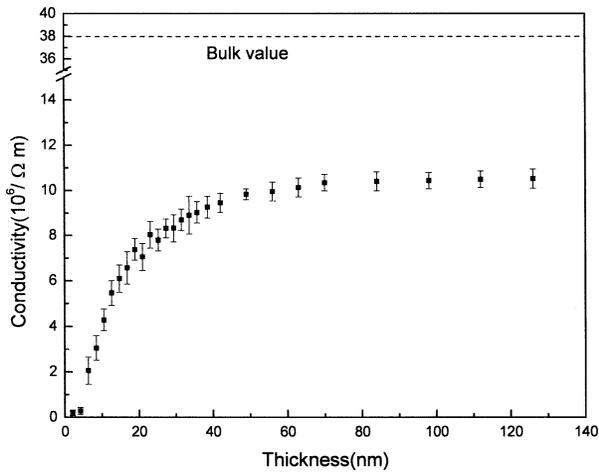
Figure 1 Thickness dependence of ultrathin aluminum films on DC conductivity.
