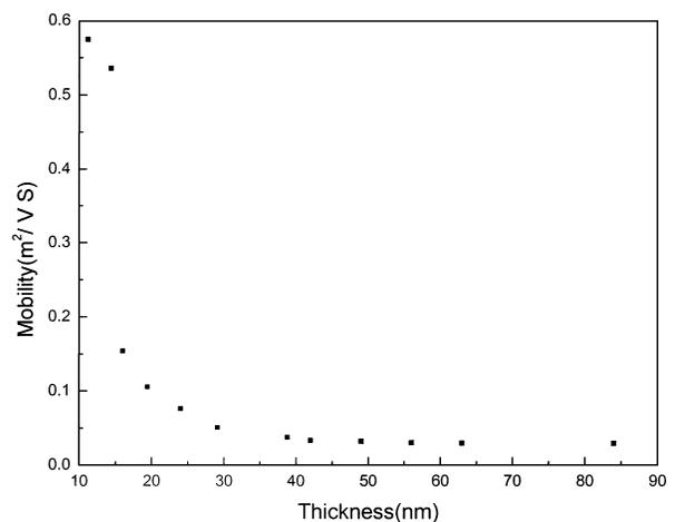
Figure 4 Thickness dependence of ultrathin aluminum films on carrier mobility.
