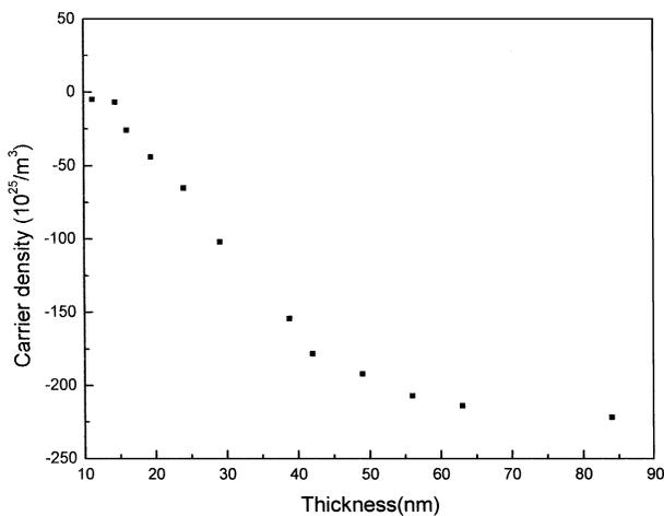
Figure 2 Thickness dependence of ultrathin aluminum films on carrier density.
